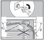
3. Set the hose correctly by loosening the ring nut.
